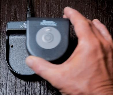
Plug power adapter into a power outlet and the base station. Place the charger in the base station. A yellow light will appear on the charger. This means the charging is in process.
