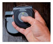
Once sufficiently charged, remove the charger from the base station. Before you place your charger in your charging collar, make sure to switch your charger on, using the circular power button in the middle of the charger.
