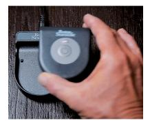
Plug power adapter into a power outlet and the base station. Place the charger in the base station. A yellow light will appear on the charger. This means the charging is in process.
